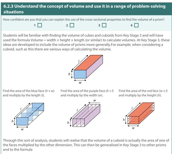
Volume of a prism = area of cross-section  $\times$  length.
